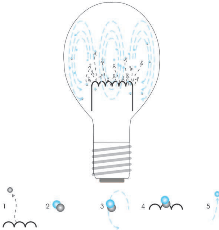
Figure 13-2 The halogen cycle extends the life of a halogen lamp. (1) Tungsten is boiled off the filament and becomes vapor. (2) Halogen gas combines with tungsten vapor to form a salt compound. (3) Convection currents circulate the compound until it comes in contact with the filament. (4) The heat of the filament breaks down the compound and the tungsten is redeposited on the filament. (5) The halogen molecule becomes free to renew the cycle.
