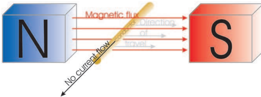
Figure 5-4 Moving a conductor in a direction parallel to magnetic lines of flux induces no current in the conductor.
