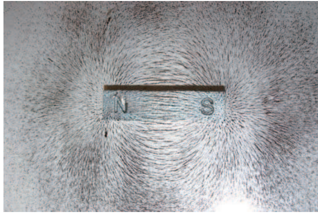
Figure 5-1 A line upon which the strength of the magnetic field is constant is called a line of flux.
