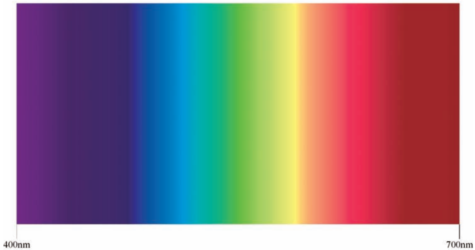
Figure 13-3 Natural visible light ranges from ultraviolet (wavelength about 400 nm) to red (wavelength about 700 nm).
