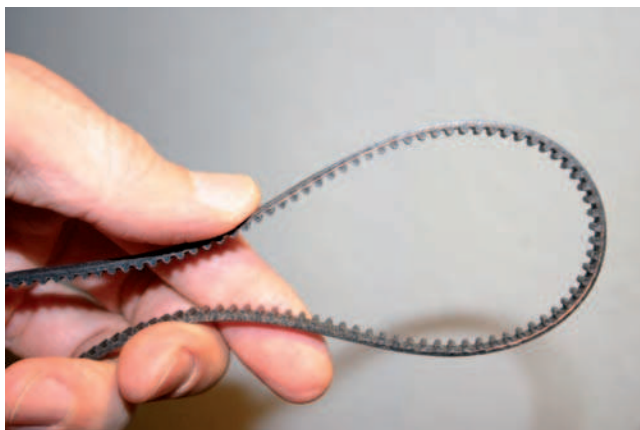
Figure 12-5 A toothed belt is functionally similar to a spur gear.
