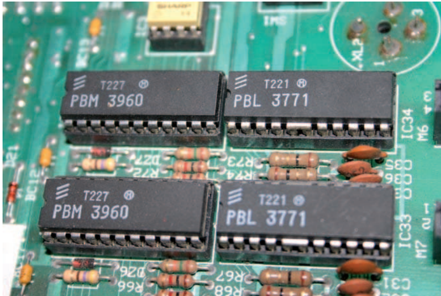
Figure 20-2 Motor drive chips supply the current to drive stepper motors. The photograph shows two PBM 3960 digital-to-analog converter (DAC) and PBL 3771 motor driver pairs.
