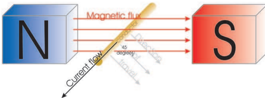
Figure 5-5 Moving a conductor at an angle relative to magnetic lines of flux will induce a current due to the perpendicular component of movement.
