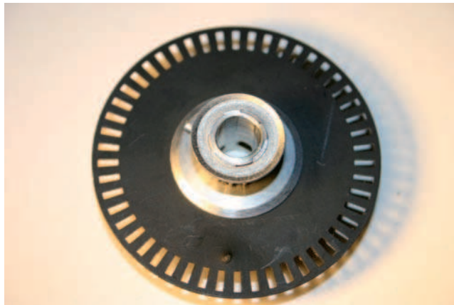
Figure 11-16 This encoder wheel works with optical sensors to locate the angular position of a stepper motor. It feeds position information back to the microprocessor to automatically correct the position should it become misaligned. This feature is often used with pan and tilt in moving yoke fixtures.
