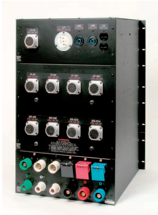
Figure 3-10 Portable power distro unit showing Cam-Lok inputs and outputs with double neutral (bottom), Socapex connector outputs (middle and top), twist-lock connectors (top), and Edison connectors (top).
