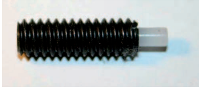
Figure 11-9 A spring plunger is sometimes used in pan and tilt systems to dampen vibrations and reduce resonance. They also increase hysteresis.
