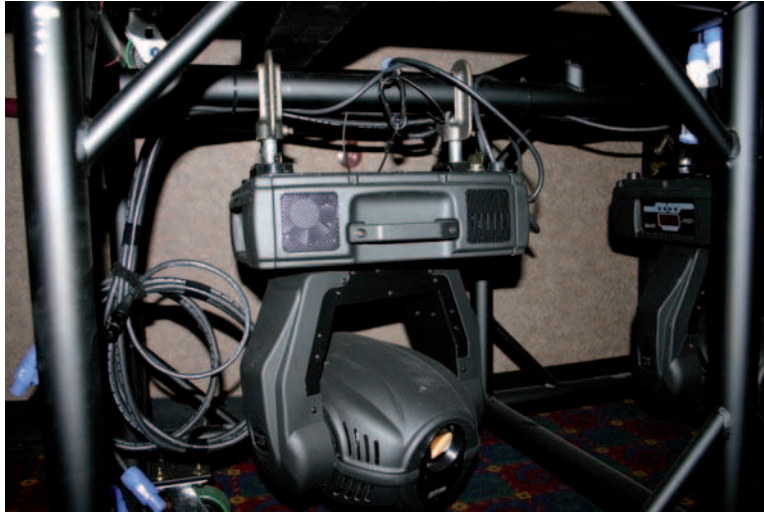
Figure 3-5 Many automated luminaries are rigged with two half-couplers.
