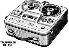
THE TELEFUNKEN KL75K has two speeds with frequency response from 60-16,000 at 3\frac{3}{4} i.p.s. and 60-10,000 at 1\frac{7}{8} i.p.s. giving over 4 hours playing time on one Telefunken DP Tape. In lightweight Styrol case (weight 20 lb.), has push-button controls and finely adjusted magnetic heads specially aligned to give maximum fidelity at low speeds.
