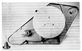
Above is the underside view of the Gramdeck, showing the large diameter plate which sits on the gramophone turntable and provides the drive for the tape transport system. The belt drive to the tape take-up spool can be seen on the left; while on the extreme left is the cone-shaped table locating pillar.
