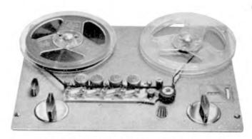
The deck with four heads fitted and cover removed.
