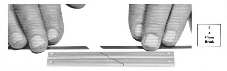
Fig. 2: A simple break, i.e., ends are undamaged and match perfectly.
