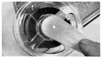
Tape rewinds at about × 3 tape speed are possible through the normal turntable drive; but faster rewinds can be achieved by hand. For this purpose a small plastic "crank" is provided, with a finger hole at the end.
