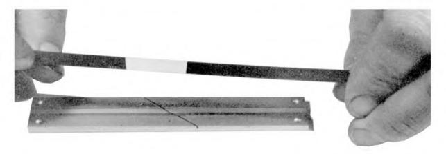
Fig. 7: Inspect the completed joint-no gap should be visible between the ends.
