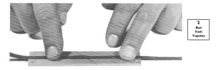
Fig. 3: Butt ends together in editing block, uncoated (glossy) side uppermost.
