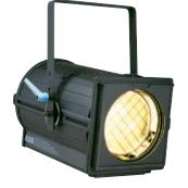
C2038° - 58°Prism-ConvexThis spotlight, based on high efficiency optics, produces a semi-sharp-edged<br/>beam. It can be used for top, front or side lighting.Field angle adjustable from 8° to 58° (4.5° - 54° beam angle).
