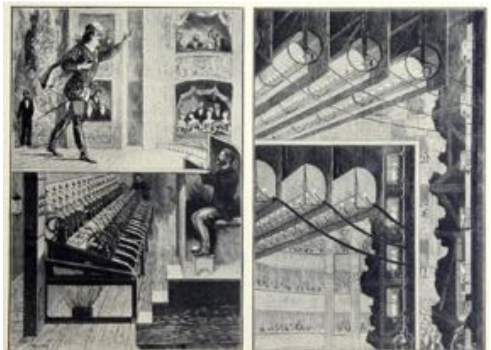
Figure 21—The electric lighting and control system used in the Paris Opera and described in L'illustration, June, 1887. The inset shows the comparison between electric and gas button lights and wing lights. The dimmers are extremely interesting. It will be noted that the discolors are mounted below the floor, and the leads brought up to contact buttons, connection to which is manipulated by means of lever arms. These lever arms can be adjusted independently or locked to a master shaft which is operated from the end by hand.
