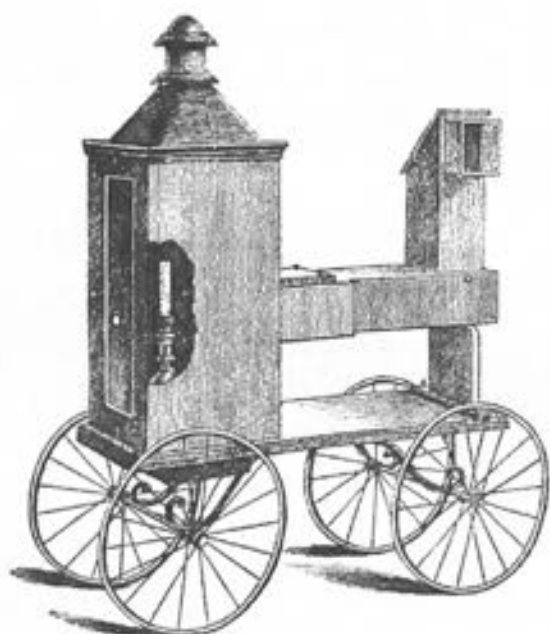
Figure 15. Weber's illumination photometer
