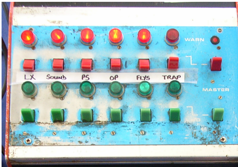
Figure 5.5.5: Early electronic prompt desk, manufacturer unknown, c1960.
