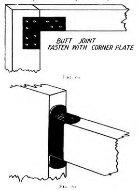
high, however, there are objections to this method. The larger the frame, the greater are the strains on the joints, and the butt joint is weaker than either of the other two I have mentioned. Consequently, I recommend the half check for scenery over, say, 10 ft. or 11 ft. in height.
