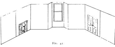
drawn, not roughly, but accurately. Mouldings, panels, etc., must be shown. Do not, however, draw anything in perspective. Where any feature projects from the wall, as, for example, a mantelshelf, draw a line to indicate where the shelf will come, cut out the shelf to scale from another piece of cardboard, and fix it in position with adhesive tape. Draw in the picture moulding, and skirting,
