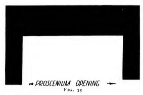
size of the actual box is not important, provided that the opening is correct to scale, in each direction. Next, mark off, on the bottom of the box, the ground plan of the stage. Then paint the surrounding part black, leaving the stage itself white (Fig. 35). You will thus obviate making use of a part of the stage that is not there! You will also be able to check the dimensions of the model when you come to put it in the box.
