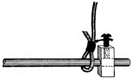
Fig. 37. Spindle of Electric Fan fitted with Spicial Collar, and Method of Securing Electric Wire Striker
