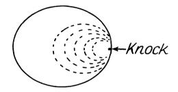
the side of the tank you will set up a wave travelling outwards but getting feebler and feebler as it gets away from the knock. Every word spoken is a knock on the atmosphere. Air waves in decreasing volume carry the sound so far, and when the wave strikes on the ear drum of the auditor, natural processes turn the air wave into sound and sound is transformed to speech.
