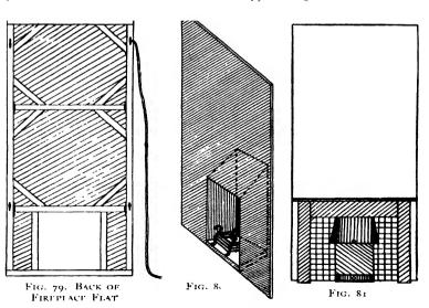
wood. Plywood can be used for the canopy and the grate. The sides of the frame are canvased and the tiles are painted.
