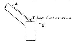
Fig. 43. Principle of Trap Doors and Briaking Joint
