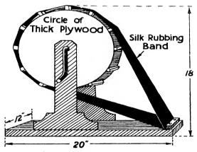
FIG. 16. PORTABLE WIND MACHINE
