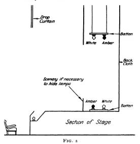
lamps in the top batten are immediately over the amber lamps in the bottom batten (Fig. 2). The effect of lightning is obtained by a rapid, alternate switching on and off of the lights. If it is impossible to obtain amber lamps the illusion may be conveyed by a rapid flickering of a row of white lamps with the stage suitably darkened. This effect is not to be recommended, but it is still
