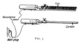
hinged as shown and kept open by a spring. The ends of the wood carry a carbon and an iron plate, and the effect is obtained by holding the apparatus in the hand and compressing it until contact is made. The length of the flash is determined by the time contact is maintained. This apparatus should be made by an experienced person and
