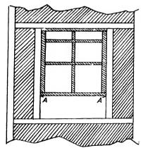
Fig. 75. Part of the Back of a Window Flat With frame of an open window fitted A -- nails supporting window frame
