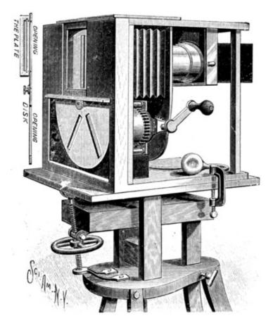
FIG. 4.—CHRONOPHOTOGRAPHIC APPARATUS PRODUCING UPON ONE PLATE A SERIES OF PHOTOGRAPHS AT EQUAL INTERVALS OF TIME.
