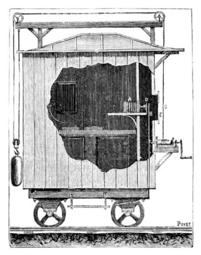
FIG. 7.—INTERIOR ARRANGEMENT OF THE DARK CHAMBER.
