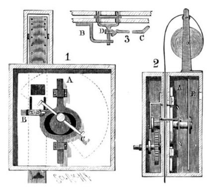
FIGS. 1, 2, AND 3.—FILM-MOVING MECHANISM.
