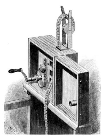
FIG. 4.—DRIVING GEAR AND FILM SUPPORT.
