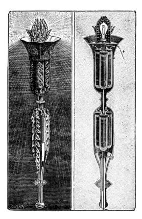
FIG. 2.—EXTERNAL AND INTERNAL VIEWS OF THE TORCH.
