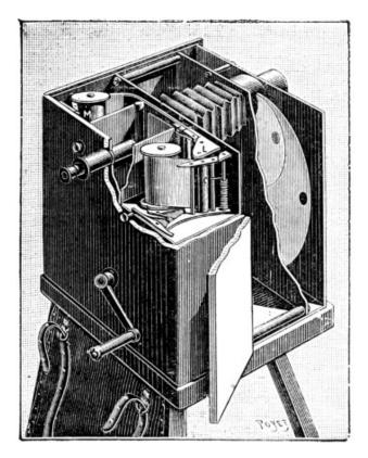
FIG. 25.—PHOTOCHRONOGRAPHIC APPARATUS.
