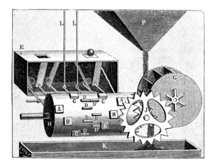
FIG. 2.—INTERNAL MECHANISM OF THE AUTOMATON.
