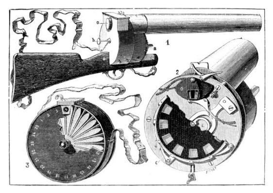
FIG. 18.—MECHANISM OF THE PHOTOGRAPHIC GUN.
