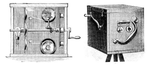
FIGS. 5 AND 6.—THE JENKINS "KINETOSCOPE" CAMERA.
