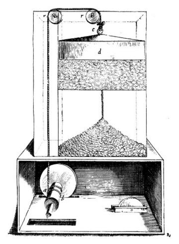
FIG. 3.—THE SHRINE OF BACCHUS. SECTION SHOWING THE PROPELLING MECHANISM.
