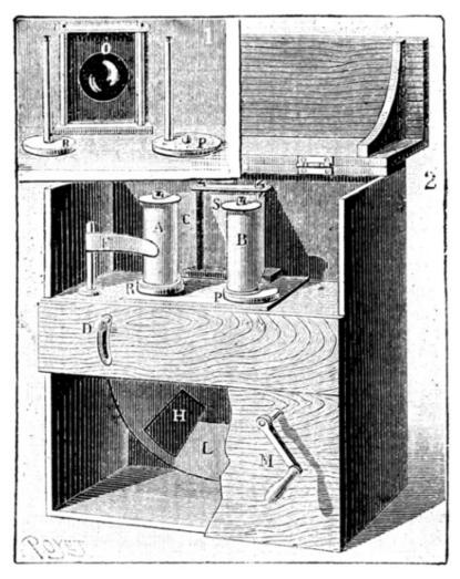
FIG. 1.—AMATEUR'S CHRONOPHOTOGRAPHIC APPARATUS.
