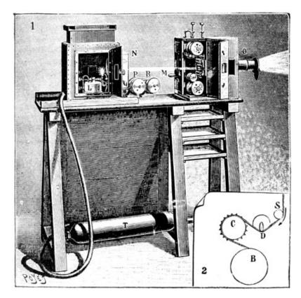
FIGS. 1 AND 2.—THE DEMENY PROJECTION APPARATUS.
