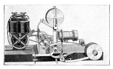
FIG. 4.—FILM PROJECTING APPARATUS.
