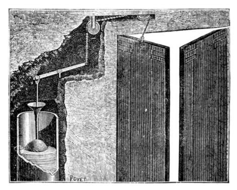
APPARATUS FOR SOUNDING A TRUMPET WHEN THE DOOR OF A TEMPLE WAS OPENED.
