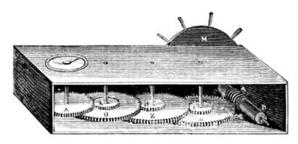
FIG. 2.—ODOMETER FOR VESSELS.
