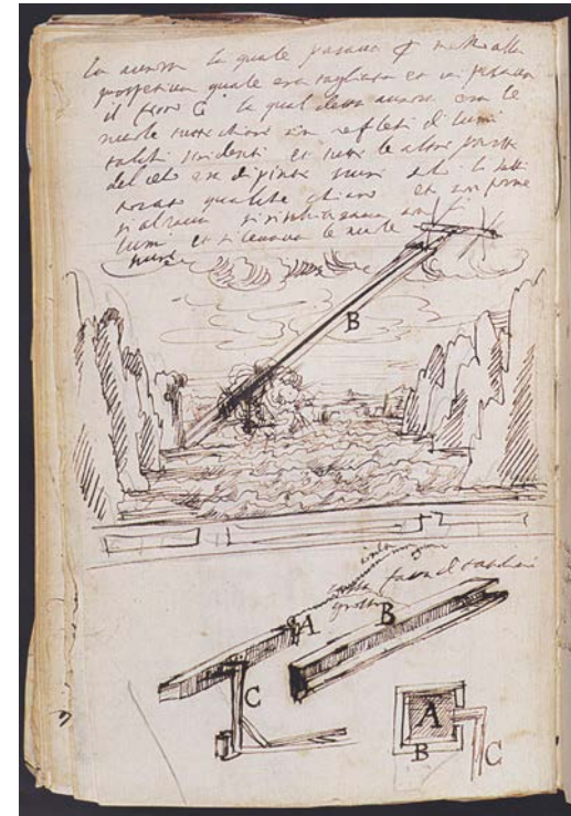
Figure 8.8 Sketch by Floriani for the mechanism by which Aurora rises in her chariot diagonally across the scene. The vehicle is carried by a hook C attached to an anima, A, running in the cassa, B. A winch at top right pulls the anima upwards. The sea is created with wave devices. Associazione Compagnoni Floriani di Villamagna. All rights reserved ©.
