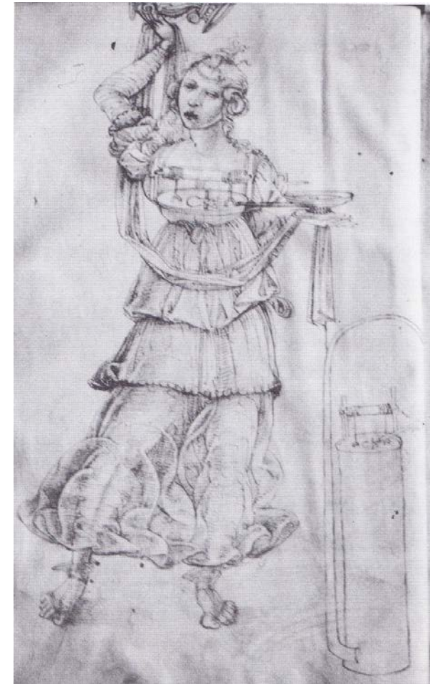
Figure 7.24 Automaton servant, shown in a drawing by Francesco di Giorgio, who pours water from a jug into a cup. The mechanism inside her chest moves her arms. At lower right is the hydraulic machinery shown removed from her body. By kind permission of the Biblioteca Nazionale Centrale, Firenze.
