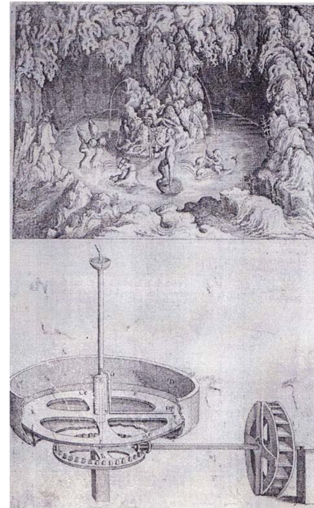
Figure 5.21 Fountain and automata in a grotto designed by Salomon de Caus. Neptune, his Tritons and attendant dolphins circle around a pool. The turntable mechanism sunk in the pool is illustrated below. From Causes of Moving Forces .
