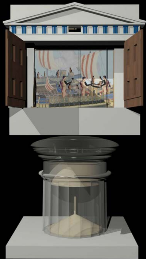
Figure 3.2 Working digital model of Hero's fixed theatre. The doors in the temple front open and close to reveal the scenes. The weight-driven motor can be seen in the pedestal. Dry sand running out into the hopper below lets the weight fall slowly. This scene from The Legend of Nauplios shows Greek boatbuilders at work. By kind permission of Richard Beacham and Janis Atelbauers.
