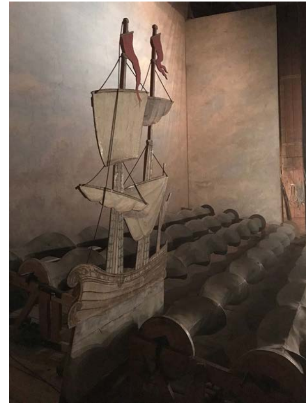
Figure 8.19 Wave machine at the Slottsteater at the Royal Palace of Drottningholm near Stockholm. The cut-out boat moves along a track. By kind permission of Drottningholms Slottsteater.
