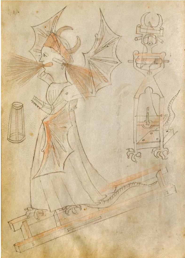
Figure 4.17 Design for a strega infuocata or ‘flaming witch’ by Giovanni Fontana, early fifteenth century. The mechanisms for moving the horns and bat wings, and for launching a bomb from under her skirt, are shown diagrammatically at the right. By kind permission of Bayerische Staatsbibliothek, Munich.
