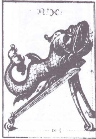
Figure 4.7 Joseph Furttenschach's design for the whale in his play about Jonah. The creature is pushed along between the waves on its trolley. The jaws are opened with a cord.
