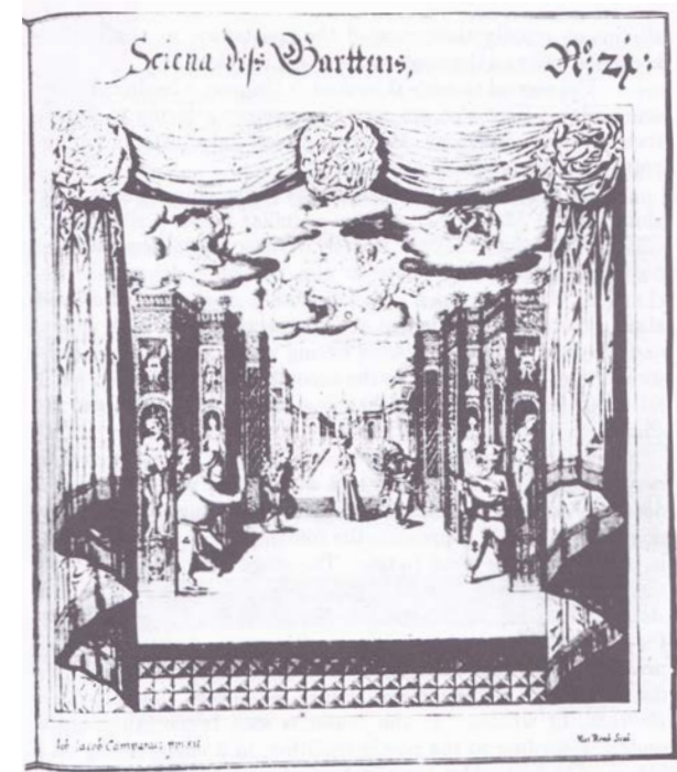
Figure 1.19 Furttentbach's drawing of his second scene, 'The Pleasure Garden', from the comedy described in Recreational Architecture : three periakttoi on each side of the stage are clearly distinguishable (compare the plan of Figure 1.18).
