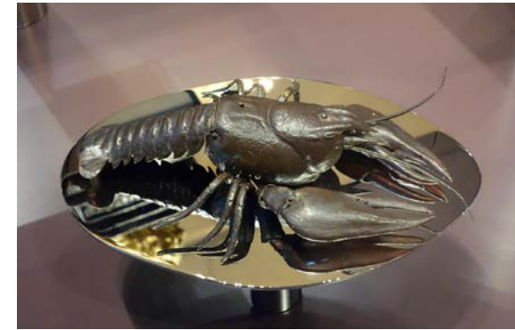
Figure 4.10 Mechanical ‘walking’ lobster made by Hans Schlottheim of Augsburg in 1589, now in the Staatliche Kunstsammlungen museum in Dresden. The creature runs on wheels and is powered by clockwork: it also opens and closes its claws. Photo: Alamy.
