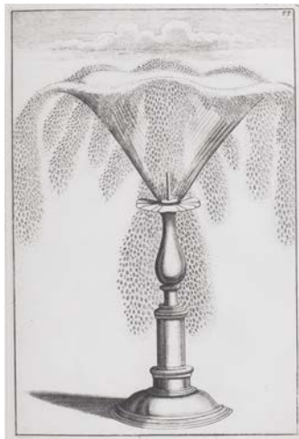
Figure 5.27 A 'morning glory' or 'trumpet' fountain designed by Georg Böckler, presumably produced with a conical plug attachment as in Figure 5.24c . From New and Curious Architecture .
