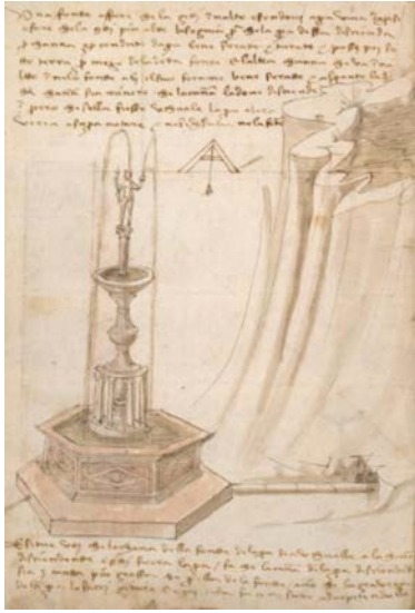
Figure 5.2 Drawing of a fountain by Mariano di Jacopo, known as Il Taccola, fifteenth century, showing water supplied from a reservoir (right) at the height of the fountain's jet. The A-shaped object to the right of the fountain is a surveying instrument for measuring the levels of reservoir and jet. By kind permission of the Biblioteca Nazionale Centrale, Firenze.
