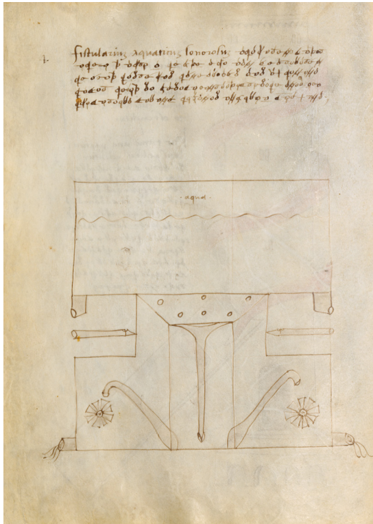
Figure 6.19 ‘Flute sounded by water’ from Fontana’s Book of Military Machines . This closely resembles the hydraulic part of the Banū Mūsà’s flute automaton with its two aeolic chambers (compare Figure 6.15 ). By kind permission of Bayerische Staatsbibliothek, Munich.
