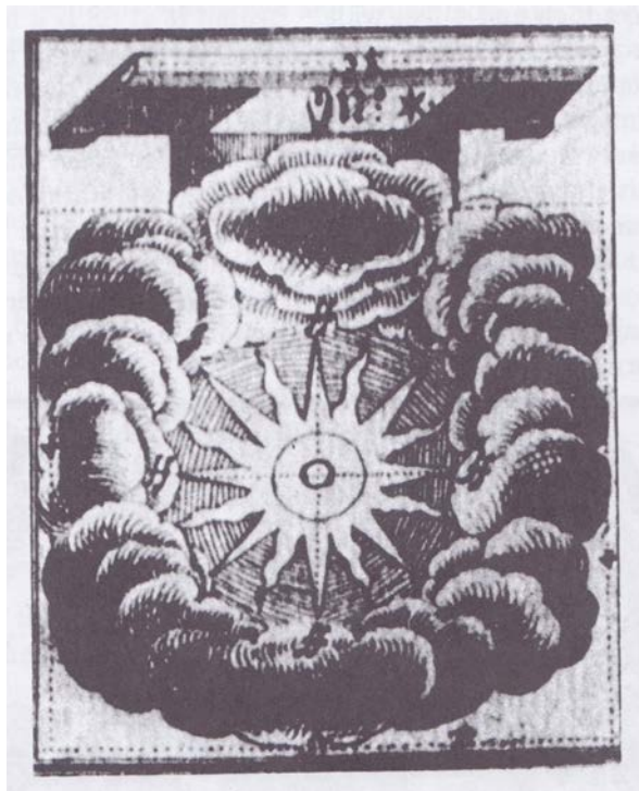
Figure B.3 A ‘glory box’ designed by Joseph Furttenbach to simulate the sun on stage. Sunbeams made of polished brass are rotated in front of a glass globe filled with water, lit by several lamps. The box is lined with gold tinsel.
