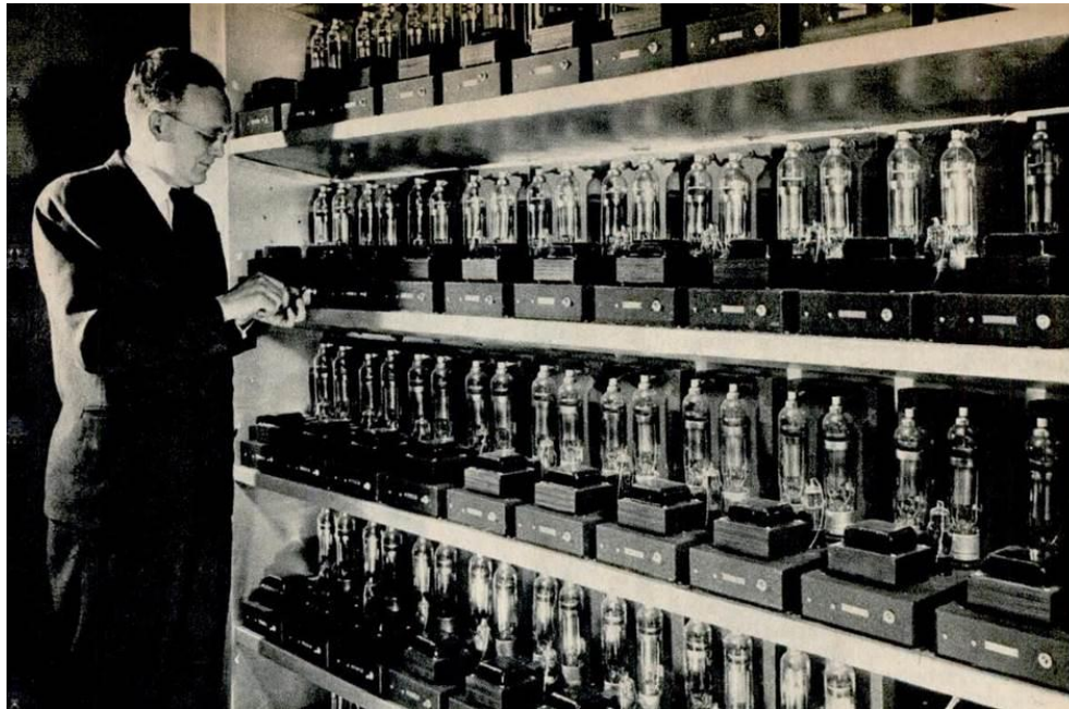
Figure 44. Professor George C. Izenour with the 44 Yale thyatron dimmers (1947)
