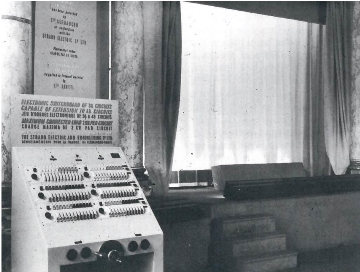
Figure 4. Electronic 36 channel demonstrator at I.T.I. Paris, 1950 (Bundy 1983)
