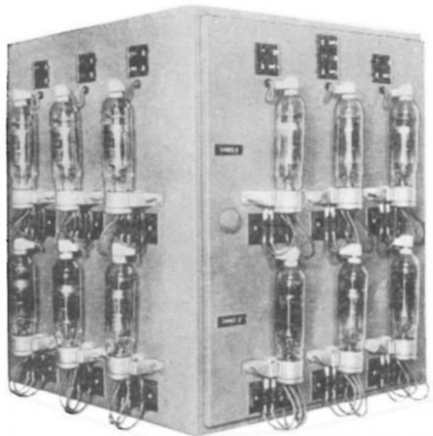
Representative cubical of Kliegtronic Dimmer Bank with six 2.5 KW dimming circuits in a 24" cube.
