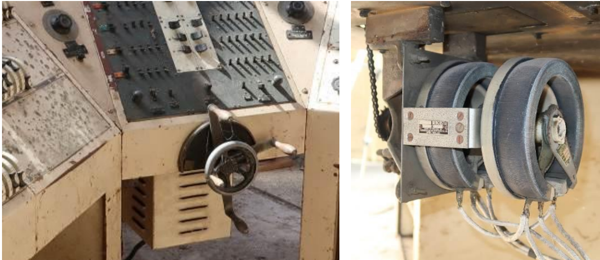
Figure 28. (left) Crossfader housing and (right) internal potentiometers
